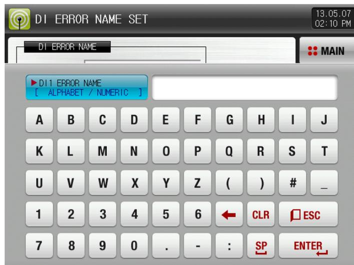
[Pic. 19–7] The setup screen parameter for display name in occurrence DI
