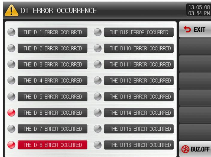
[Pic. 7-3] The screen with letter for DI error display method
