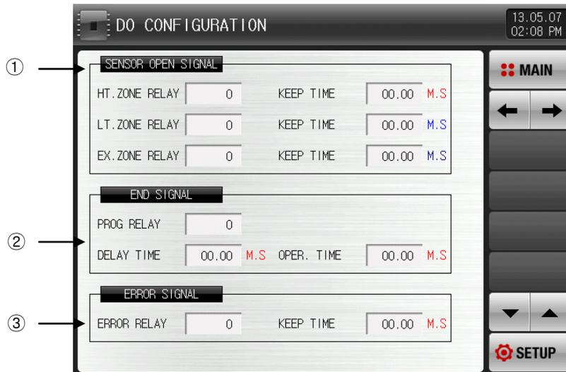
[Pic. 18-8] The second screen for other signal relay setup
