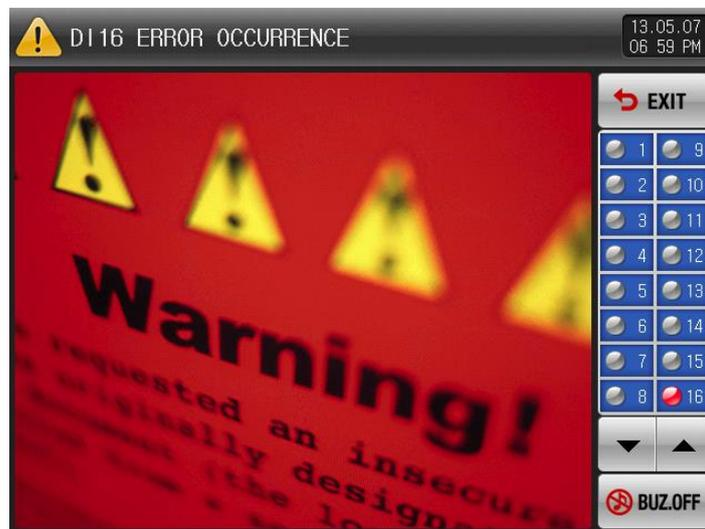
[Pic. 7-4] The screen with photo for DI error display method
