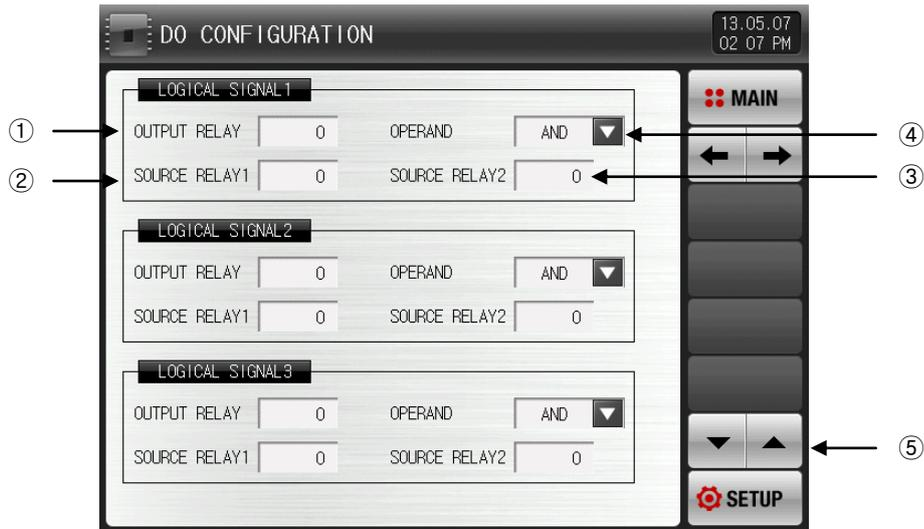
[Pic. 18-5] The setup screen for logical signal
