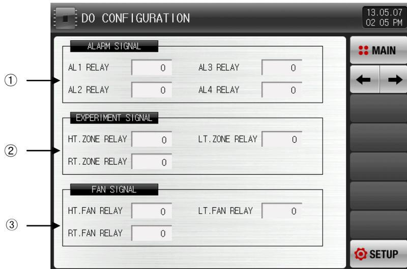
[Pic. 18-2] The setup screen of alarm signal/experiment signal/fan signal relay
