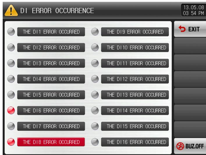
[Pic. 19-12] The screen with letter for DI error display method
