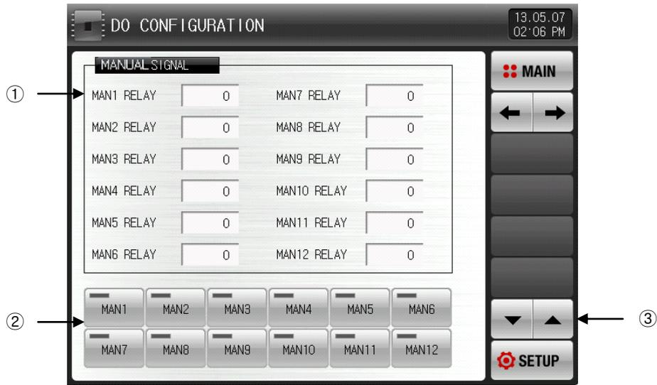
[Pic. 18-4] The setup screen for manual signal
